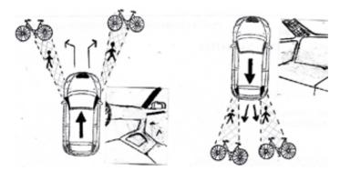
Remember that certain parts of the **chassis** create blind points and reduce the visibility: creating an obstacle between you and the object in all directions: forwards and backwards, to the right and to the left.
