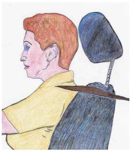
The headrest serves to avoid or to diminish damages at the cervical column, that is a WHIP OF HIT during an accident, specifically during a rear end collision.
